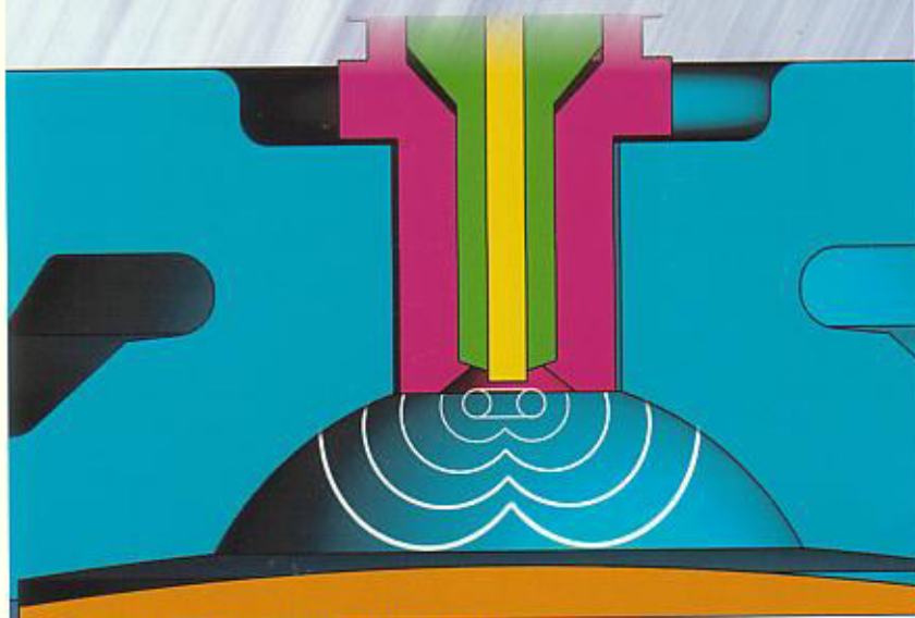
FIG 8/6 EXPANSION DE LA COMBUSTION
